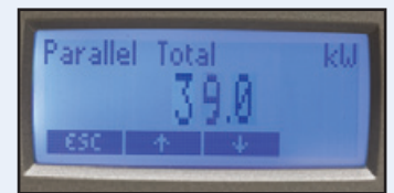
Display full system output from any UPS
