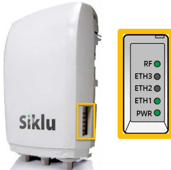
Figure 5: MultiHaul™ B100 - front view and LEDs
