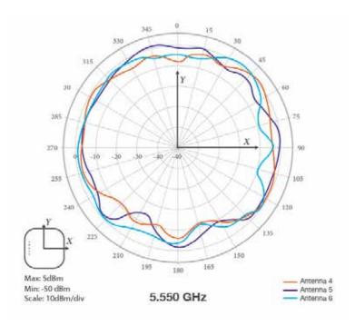
**Horizontal or Azimuth (Top View)**
